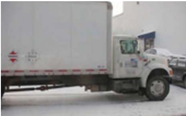
Good Practice: A hazardous materials transport truck with appropriate placards and signs.
