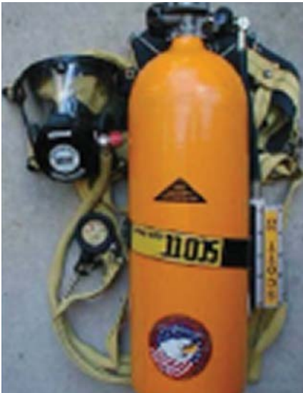
SCBA for emergency or planned entry into unknown concentrations or IDLH (Immediately Dangerous to Life or Health) conditions
