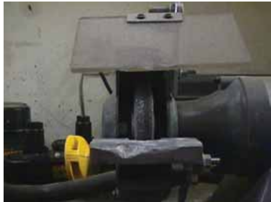
Good Practice: Grinding wheel with eye shield in place
